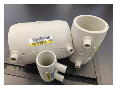
With the application of our **PP electric-wielding sleeves**, a workshop prefabricated assemblies, developed from sketches, can be joined to existing lines without using butt welding machines, which are typically cumbersome, heavy and difficult to use at heights or in plants where multiple pipelines are positioned close together.
